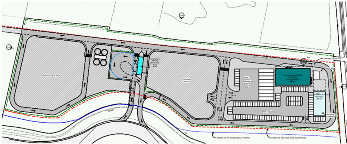
Figure 67. Overall Site Plan - South Terminal Roundabout
